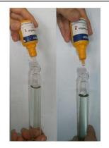
1. Add 5 ml of sample to the test tube. Add 7 drops of Reagent 1 and 7 drops of Reagent 2. Cap, then invert the tubes several times. Water turns light pink or light yellow, then light green or blue if sulfide is present.
