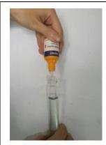
2. Wait 3 minutes. Add 7 drops of Reagent 3. White precipitate forms. Shake well until the precipitate completely dissolves.
