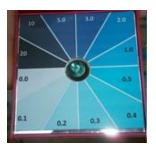
**4**. Find the best matched color. Record total sulfide level. Look at the Table 1 for the threshold of total sulfide for shrimp ponds. Look at Table 2 for the percentage of free  $H_2S$ .
