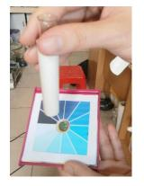
3. Place the tube into the comparator. Remove the cap. Hold the comparator with tube top pointing light source and tube bottom reflected in the mirror on the color chart as shown in the figure
